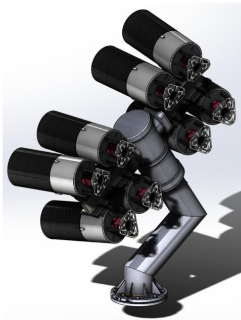
Fig2. INF multiaperture telescope: 8 x VT-78d telescopes on ASA DDM160 mount.
