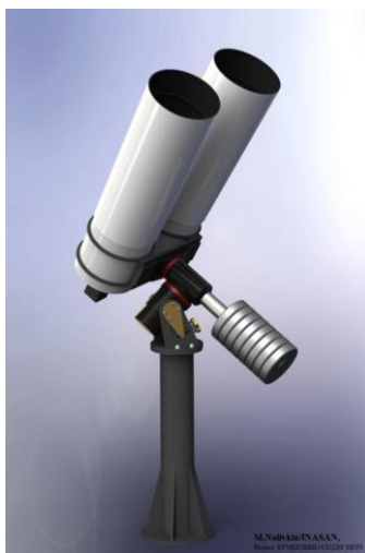
Fig9. INF prototype drawing, 2 x VT-78d telescopes on ASA DDM85PRO mount.
