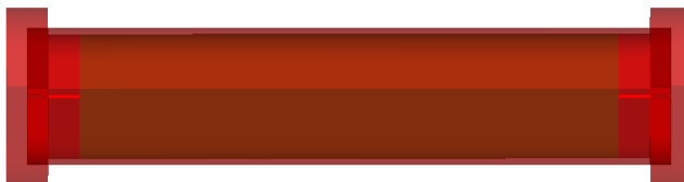
Fig2. Model of copper proportional counter. A darker color indicates the operating area of the detector.
