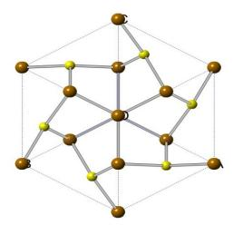
The mineral pyrite, or iron pyrite, also known as fool's gold, is an iron sulfide with the chemical formula FeS<sub>2</sub>. Pyrite has been proposed as an abundant, inexpensive material in low-cost photovoltaic solar panels. Synthetic iron sulfide was used with copper sulfide to create the photovoltaic material.
