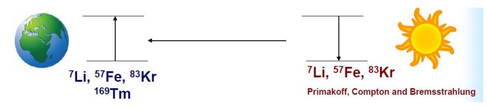
The monochromatic axions emitted by <sup>7</sup>Li, <sup>57</sup>Fe and <sup>83</sup>Kr nuclei can excite the same nuclide in a laboratory, because the axions are Doppler broadened due to thermal motion of the axion emitter in the Sun, and thus some axions have needed energy to excite the nuclide.
