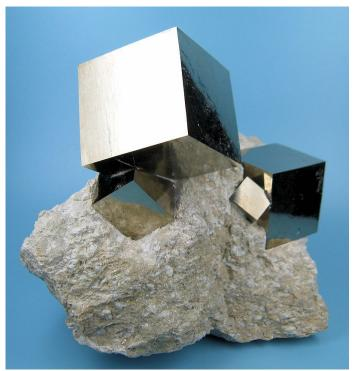
The band gap in pyrite is about 0.95 eV and the dominant charge carriers can be either electrons or holes. Sometimes, both n-type and p-type semiconducting regions can be found within single naturally occurring crystals
