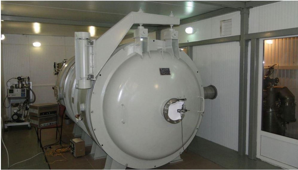
Fig5. The OGRAN detector chamber in the dust-protected box.
